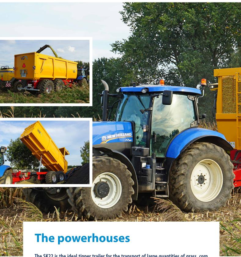
The SK22 is the ideal tipper trailer for the transport of large quantities of grass, corn and similar products. The fully welded and smooth finished load area ensures problem-free unloading. Furthermore, the rear hinge is placed more toward the centre, which creates the maximum overlap. The tipping cylinder is located in a cardanic suspension and the entire tipper trailer is perfectly finished.
