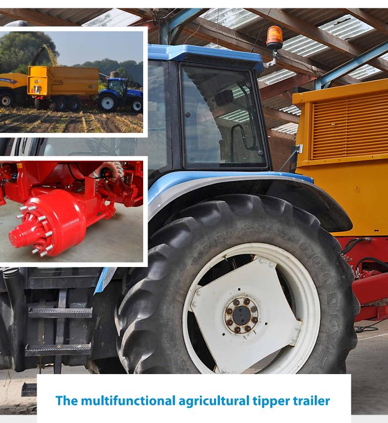
The LK 16 kipper is extremely suitable for larger quantities, but remains compact. The high tipping angle of 60° and the smooth finish of the container ensures that all products are unloaded without any problem. The grain chute in the rear tailgate has a wide unloading opening and can be operated from two sides.
